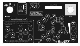
Figure 8-3. Ground Controls with Jib Rotator
